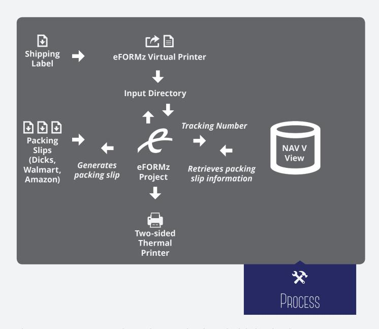
The main project extracts the tracking number from the label and makes an SQL query to the database. The retrieved information is used to generate the packing slip. The shipping label and newly generated packing slip are then duplexed and sent to the Toshiba DB-EA4D.
